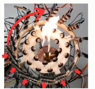
Stationary, 'pushed' flame. Active columns marked with small red arrows, rotation of active transducers marked with large red arrow.
