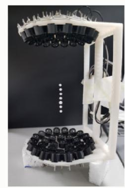
TinyLev array, built for some initial testing + Good resolution, produced large forces - Could only produce one, simple pressure field, too small to be safely used with fire
