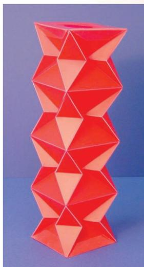
**Crush-resistant.** Pleated columns inspired by a beverage can are strong but lightweight—a combination that may prove useful in silos, rocket bodies, and shock absorbers.
