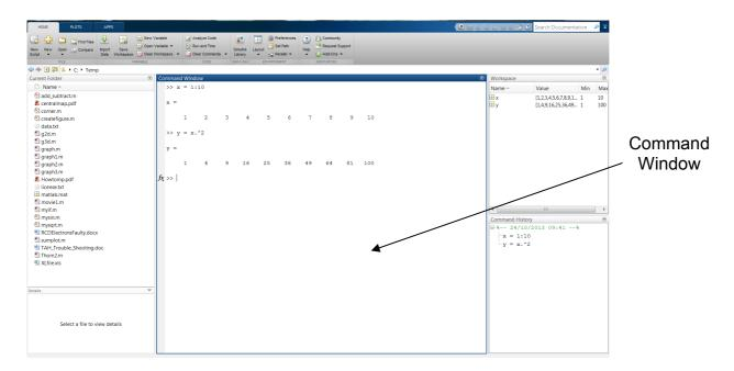
The exact layout of the subwindows does vary from version to version. It is also possible to change the layout, so the appearance may be different from the picture above. However, it should be fairly easy to find the Command Window, which is normally the largest window. Don't worry about the other windows for the time being. You will be shown how to use them later. We are going to start by entering commands into the command window.
