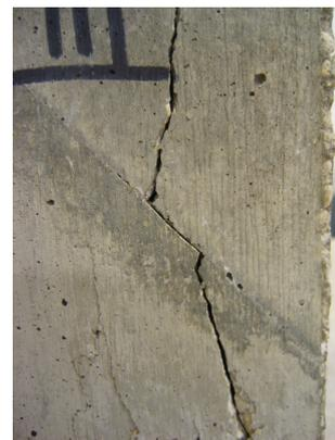
Figure A.5: Enlarged crack along joint surface
