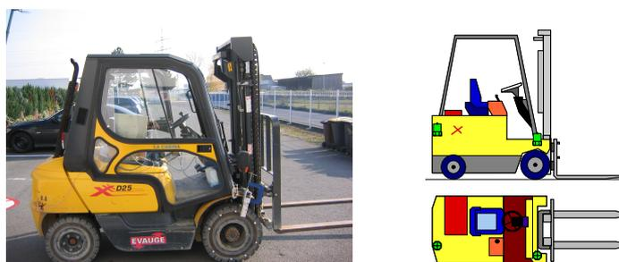
Figure 2.20: OM Pimespo XD25 and sketch of positions of accelerometers
