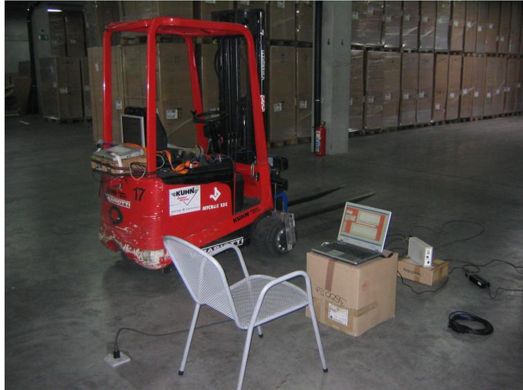
Figure 4.8: Fork-lift truck and floor set up for testing
