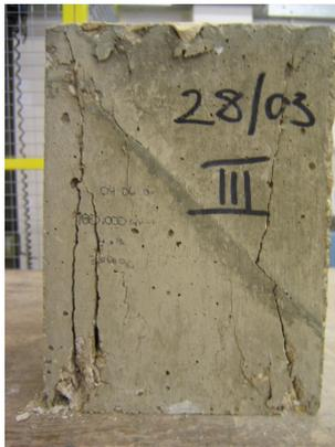
Figure A.4: Typical failure mechanism of specimen type 1
