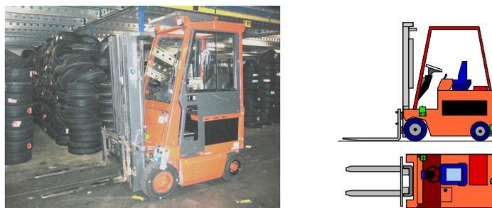
Figure 2.18: Nissan FP01 R15 and sketch of positions of accelerometers
