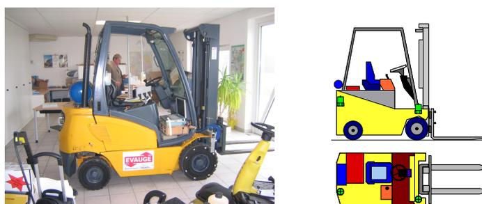
Figure 2.19: Jungheinrich TFG16 AK and sketch of positions of accelerometers
