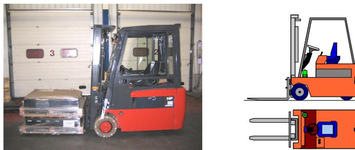
Figure 2.17: Nissan GNX 1L16HQ and sketch of positions of accelerometers
