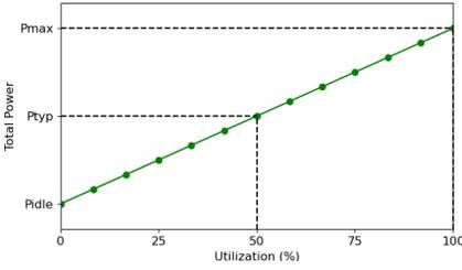
Fig. 4. A power model of a router
