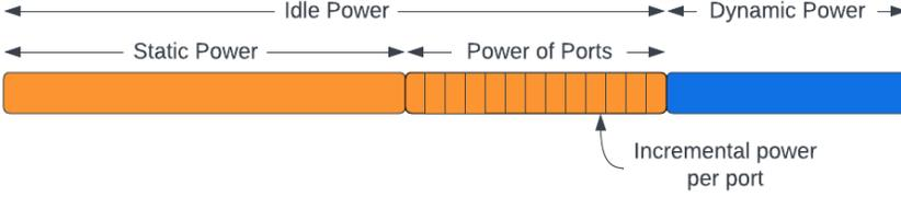
Fig. 6. A breakdown of the power components of a router: idle vs dynamic power
