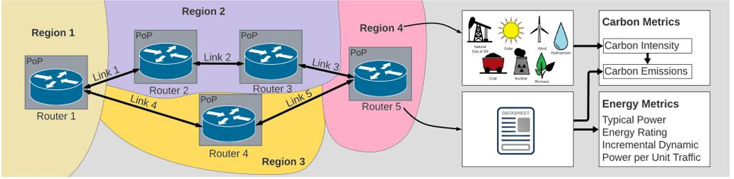
Fig. 3. Overview diagram of the system
